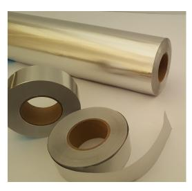
Our offer includes VaporBarier foil in two variants: basic foil - clean, and self-adhesive foil. The VaporBarier foil and tape consists of three layers: 12µ polyester foil, 25µ aluminum foil, 12µ polyester foil. The self-adhesive variant uses acrylic glue. A large temperature range from -65°C to + 150°C allows for a very wide range of applications. The main place of
